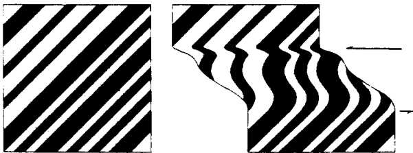
Fig. 12. Folds of 'similar' style produced by the shearing of passive layers.
